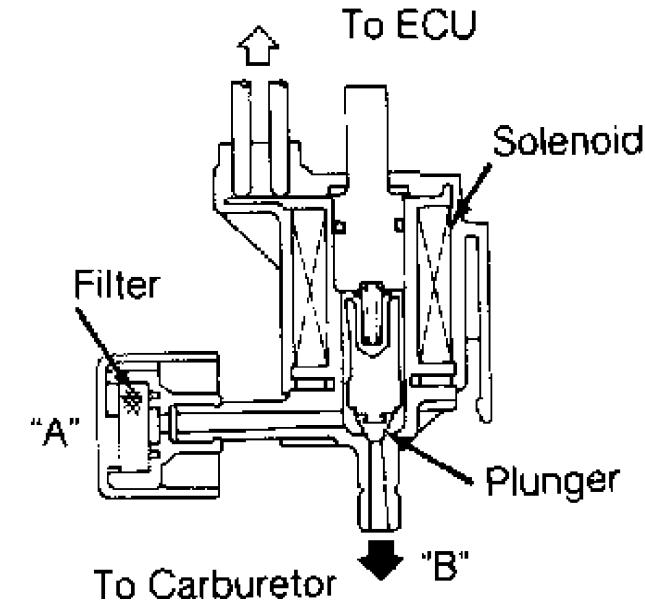
Fig. 17: Testing High Altitude & Vacuum Line Control Solenoid(s) Courtesy of Subaru America, Inc.
