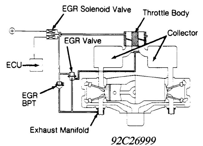
Fig. 8: EGR System (SVX) Courtesy of Subaru of America, Inc.
