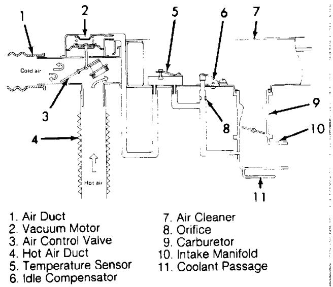
Fig. 23: Cross-Sectional View Of Thermostatic Air Cleaner (Justy) Courtesy of Subaru of America, Inc.
