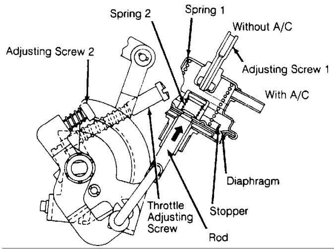
Fig. 1: Fast Idle Control Device (FICD) Control Actuator Courtesy of Subaru of America, Inc.
