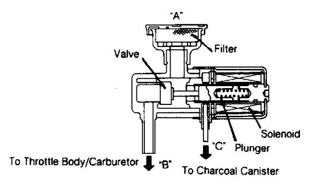
Fig. 16: Testing Bowl Vent Or Purge Control Solenoid Valve Courtesy of Subaru America, Inc.
