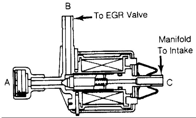
Fig. 9: Cross-Sectional View Of EGR Solenoid Valve Courtesy of Subaru of America, Inc.
