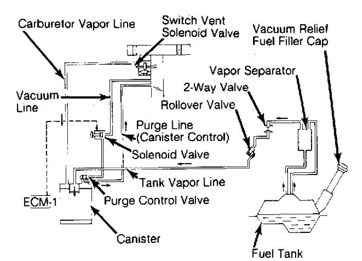
Fig. 10: Fuel Evaporation System (Justy) Courtesy of Subaru of America, Inc.
