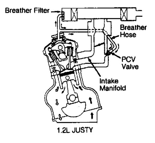
Fig. 18: Positive Crankcase Ventilation (PCV) Systems (Justy) Courtesy of Subaru America, Inc.
