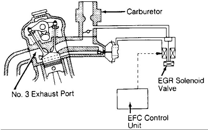
Fig. 6: EGR System (Justy Carbureted) Courtesy of Subaru of America, Inc.
