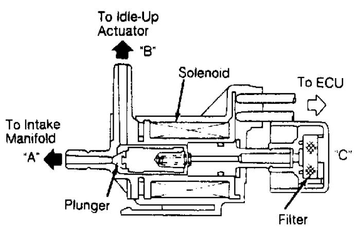
Fig. 2: Identifying Idle-Up Solenoid (Justy Carbureted) Courtesy of Subaru of America, Inc.
