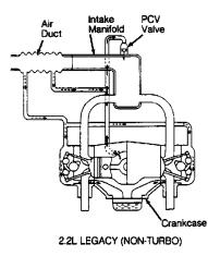
Fig. 20: Positive Crankcase Ventilation (PCV) Sys (Legacy Non-Turbo) Courtesy of Subaru America, Inc.
